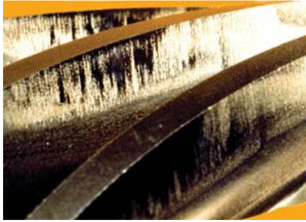
A lubricant with inadequate anti-scuff additives caused scuffing on this spiral bevel pinion.
