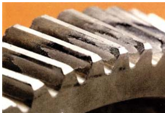
Micropitting often will have a pattern that indicates misalignment.
